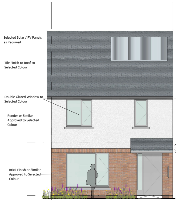
1 Front Elevation Option A, B & C (Half Brick) 1 : 100
