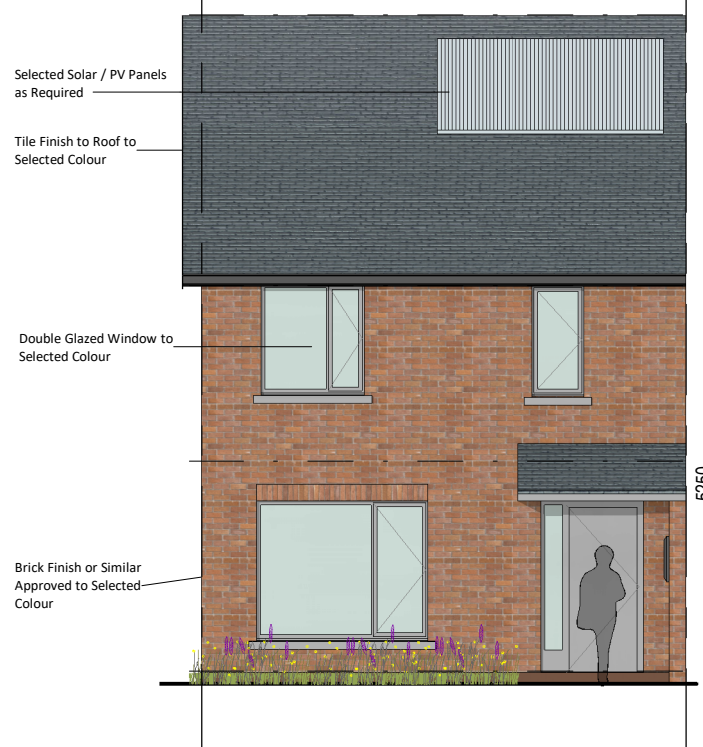
8 Front Elevation A, B & C (Full Brick) 1 : 100
